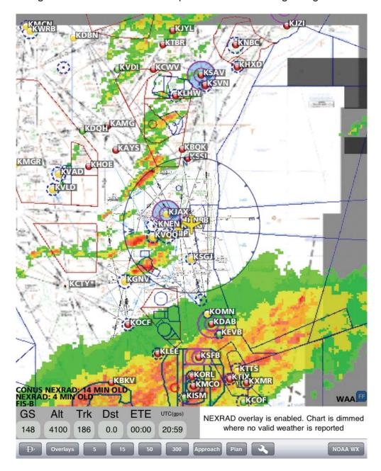
A tip to verify Stormscope or Strikefinder accuracy is to pan a NEXRAD cell under the circular icon and check the range and bearing to the cell by checking the bearing and distance panned (which shows up on a blue background at the lower right), against the bearing and range shown to the lightning strikes on the sferics equipment.
